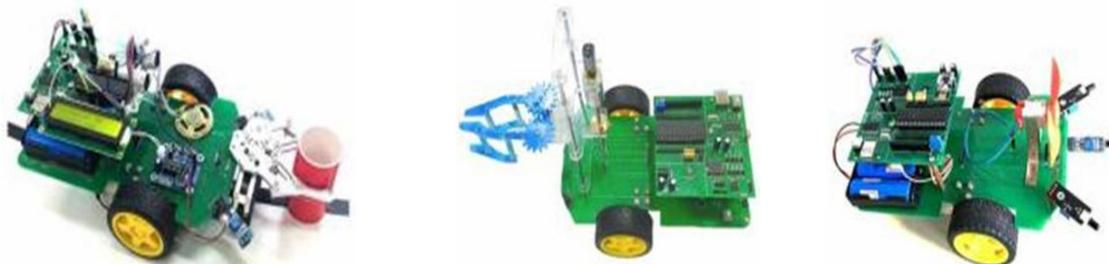
(a) Infrared and wireless handling vehicle (b) Infrared and voice control vehicle (c) Fire fighting vehicle
